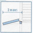
Disconnect downspouts, cap foundation drains and extend downspouts and sump discharge pipes to direct water at least 2 m from foundation
